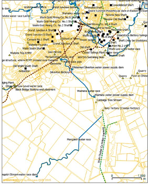
The battery, here labelled Silverton Battery, can be seen at middle (red triangle), with its associated water races in blue (the four lower water races). The tramways are designated by brick coloured dotted lines. The blank area at top middle is Martha mine, Union Hill to the right, and the black squares indicate mine shafts. The yellow lines are cadastral lines (property boundaries).
