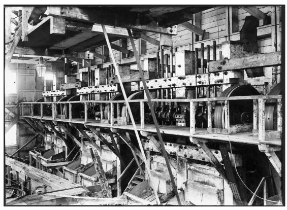
Union battery stampers. The cam shafts and bull wheels stretch across the middle of the image. Six mortar boxes are visible below.  $FL16664154\ ATL$
